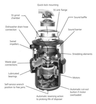
Continuous feed waste disposer - by In-Sink-Erator
